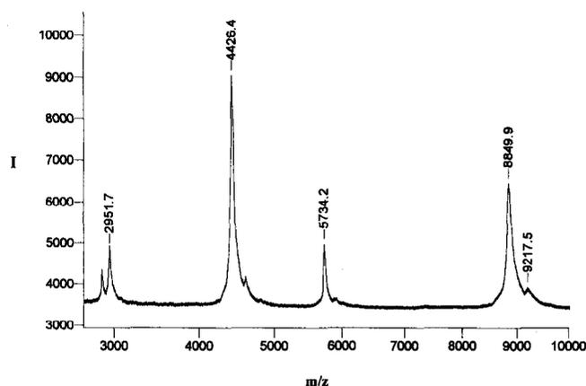
**FIG. 1.** MALDI-MS spectrum of MPIF-1d23 chemokine from CHCA matrix exhibits singly, doubly and triply charged ions at  $[M + H]^+$  8849.9,  $[M + 2H]^{2+}$  4426.4, and  $[M + 3H]^{3+}$  2951.7, respectively. Insulin is the internal standard with  $m/z$  5734.2.
