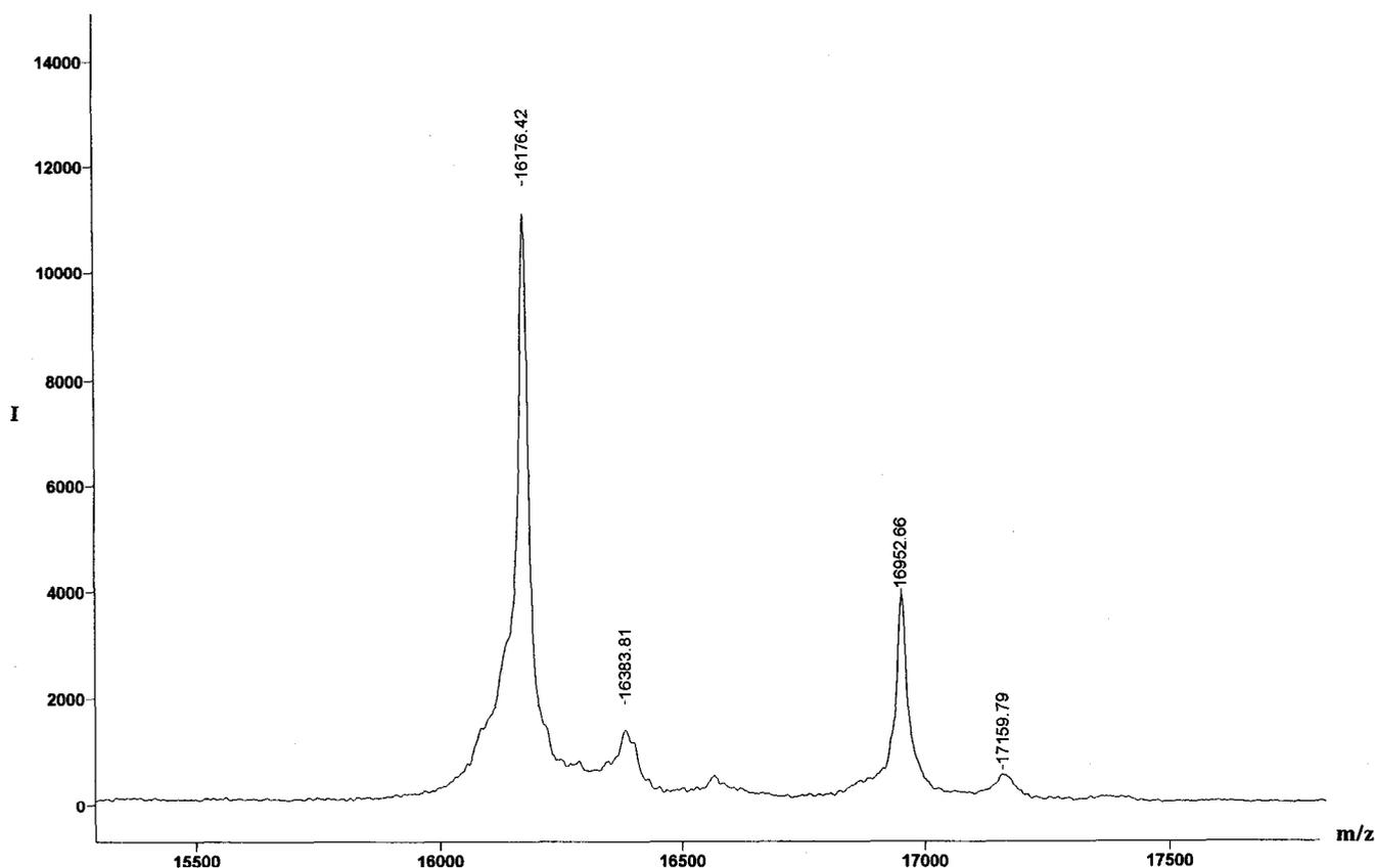
**FIG. 2.** DE-MALDI-MS spectrum of the KGF-2d33 protein in SA matrix, showing the  $[M + H]^+$  at 16,176.42 and the matrix adduct at  $m/z$  16,383.81. The internal calibration compound myoglobin is indicated by the  $[M + H]^+$  at 16,952.66, and its matrix adduct is shown by  $m/z$  17,159.79.
