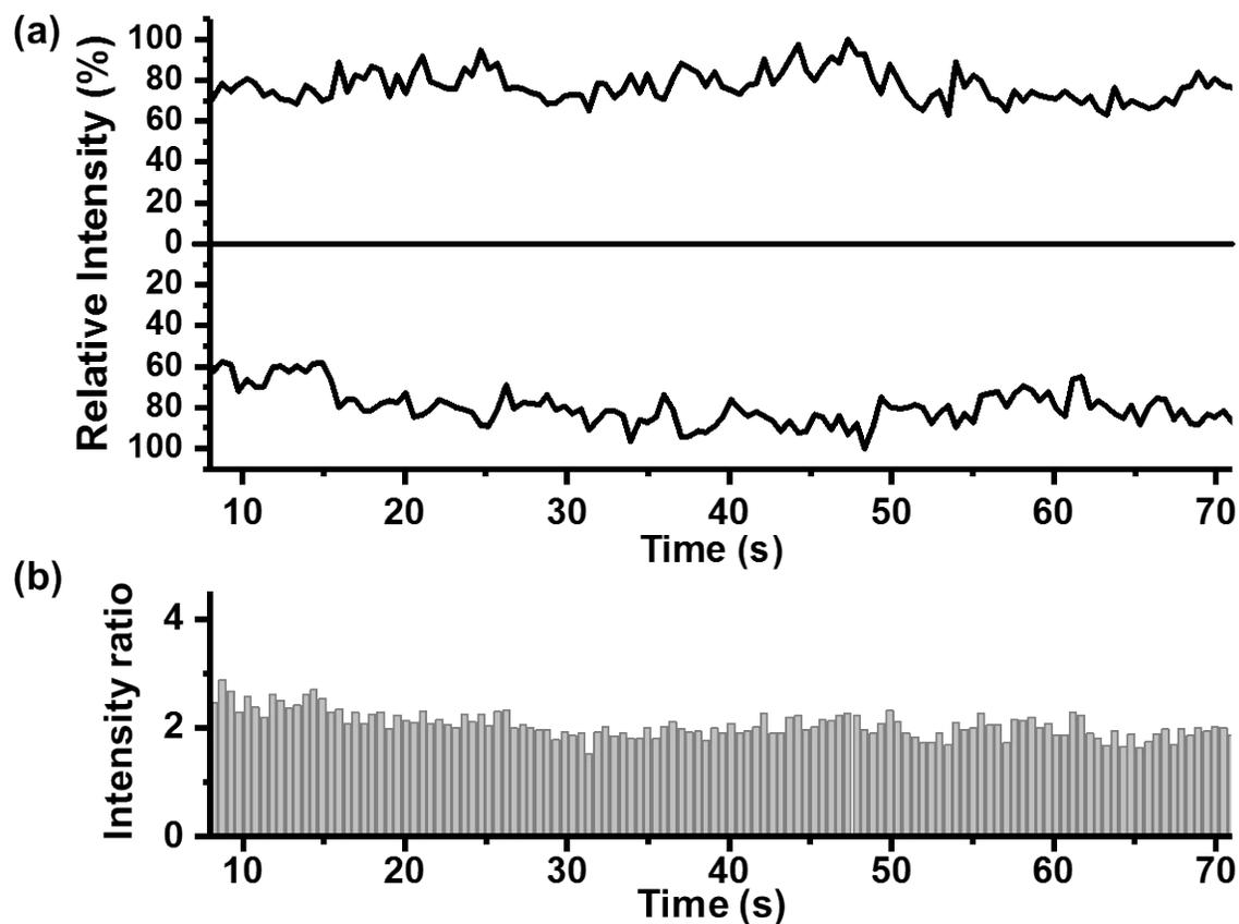
**Figure S4.** (a) Time dependence of ion intensities from two barrels of a theta capillary. Barrels are loaded with 0.76  $\mu\text{M}$  arginine at 1500 V (spray 1, top trace), and 0.20  $\mu\text{M}$  verapamil at 1000 V (spray 2, bottom trace). (b) Signal intensity ratio of arginine to verapamil (spray 1 to spray 2) as a function of time.
