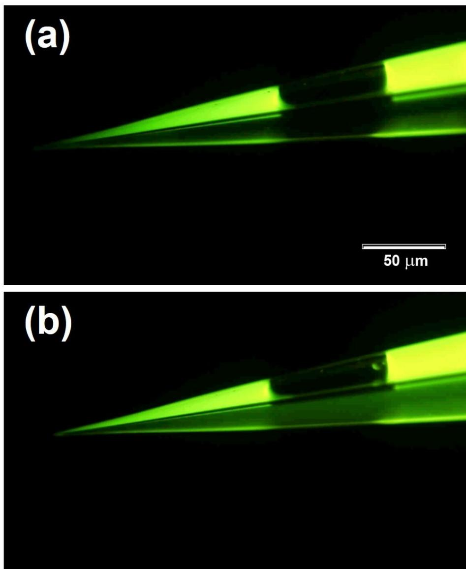
**Figure S3.** (a) Fluorescence microscope image (excitation at 470-490 nm and emission at 520 nm) of theta capillary of  $>5 \mu\text{m}$  tip diameter with barrels loaded with 6 mM rhodamine 6G and water before voltages are applied. (b) Applying 500 V and 300 V to the barrels containing rhodamine 6G solution and water, respectively, results in electroosmosis.
