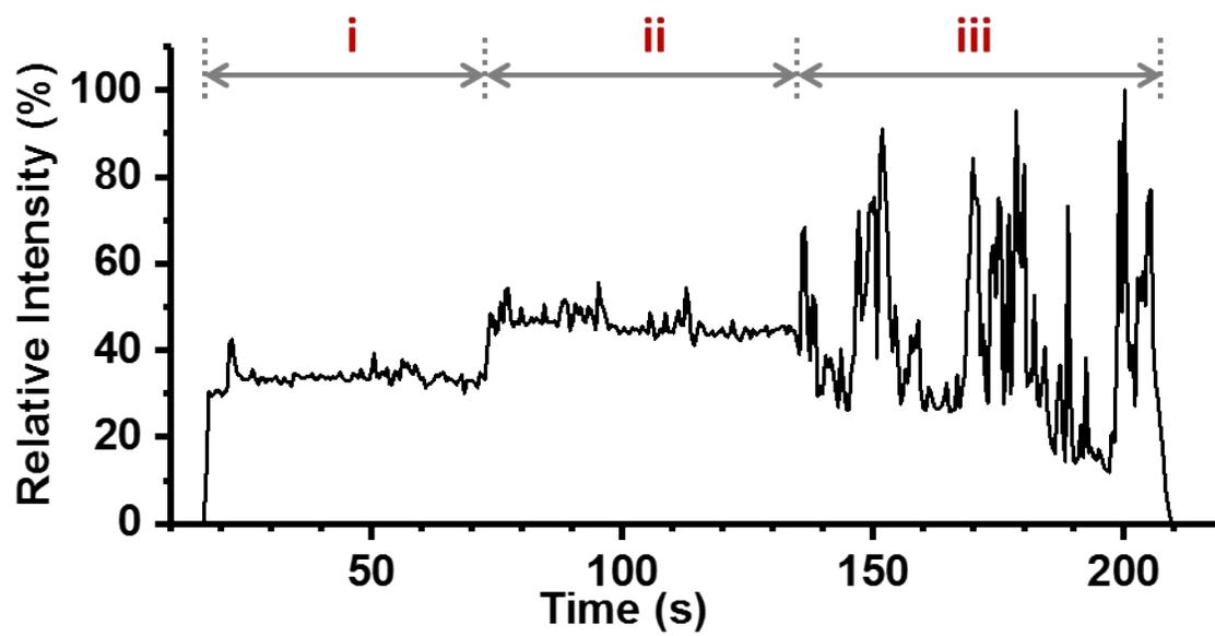
**Figure S2.** Time dependence of verapamil ion intensity showed a transition from (i) stable signal at 800 V spray voltage, (ii) through slight fluctuations at 1800 V, (iii) to a highly unstable spray at 2800 V.
