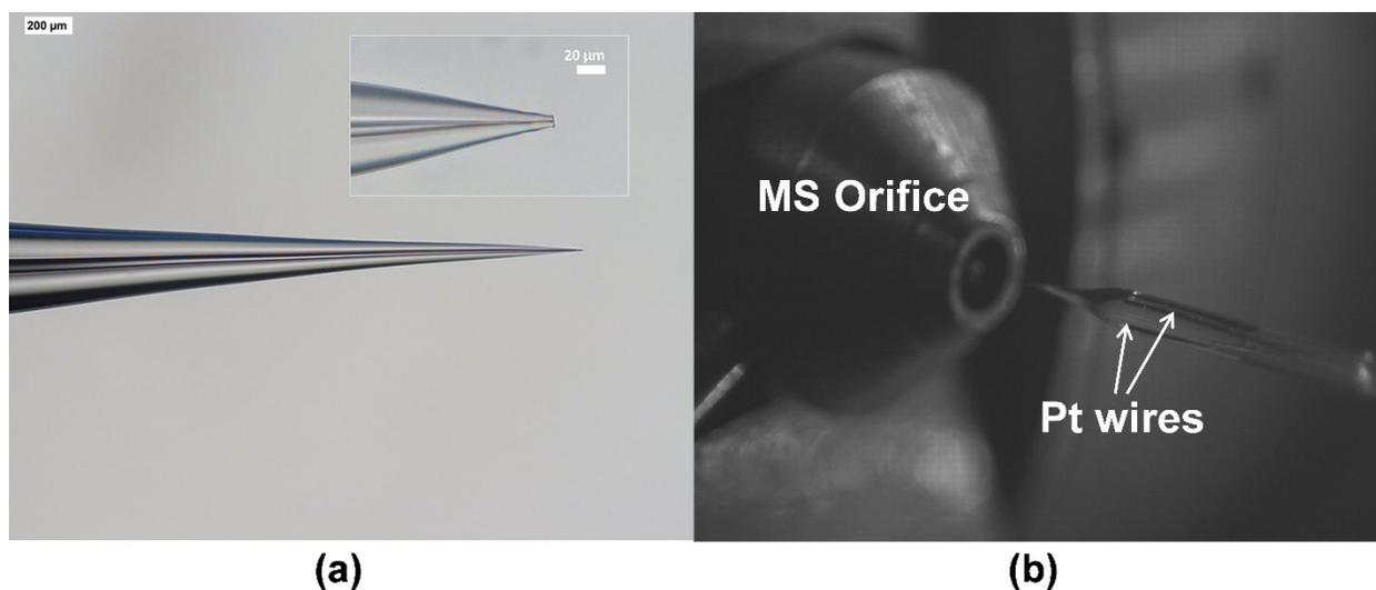
**Figure S1.** (a) Pulled theta glass capillary with a typical tip diameter of  $\sim 3 \mu\text{m}$ . Image in the inset at higher magnification shows a larger tip diameter of  $\sim 8 \mu\text{m}$  with a  $\sim 1 \mu\text{m}$  wide septum that reaches the tip of the capillary. (b) Pulled theta glass capillary in front of the mass spectrometer inlet orifice with two platinum wire electrodes inserted for generating gradient electrospray.
