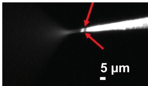
Fig. 4 Microscope image of spray geometry formed at two barrels of a theta capillary with static voltages of 1800 V and 2200 V applied. Two separate liquid filaments were formed, indicative of two Taylor cones.
