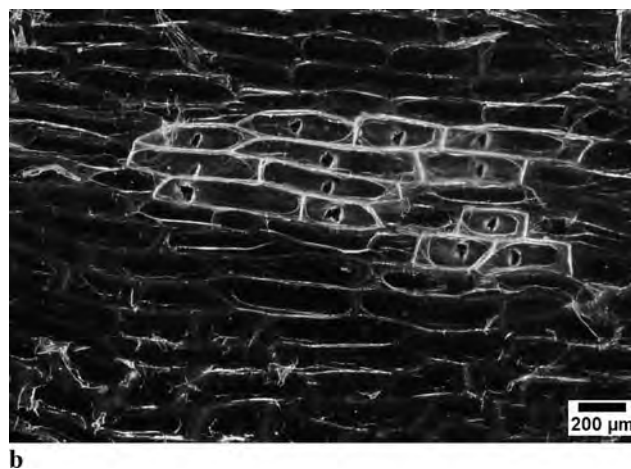
Fig. 1 (a) Schematic representation of the laser ablation geometry for energy deposition through a sharpened optical fiber. Parameters D , R , \theta , and d stand for the optical fiber core diameter, the etched tip radius of curvature, the angle of inclination, and the distance from the tissue surface, respectively. (b) Ablation marks on single adjacent A. cepa cells
