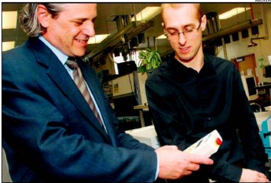
Akos Vertes (L), professor of chemistry, biochemistry, and molecular biology, and graduate student Peter Nemes show their detector, which combines a laser with a mass spectrometer to provide on-the-spot analysis that researchers hope will have applications ranging from evaluating a tumour as it is removed to quickly detecting explosives in luggage
