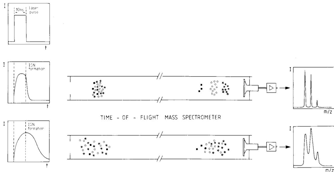
**Fig. 1.** Effect of the time-definition of the ion formation process on the mass resolution in LMMS
