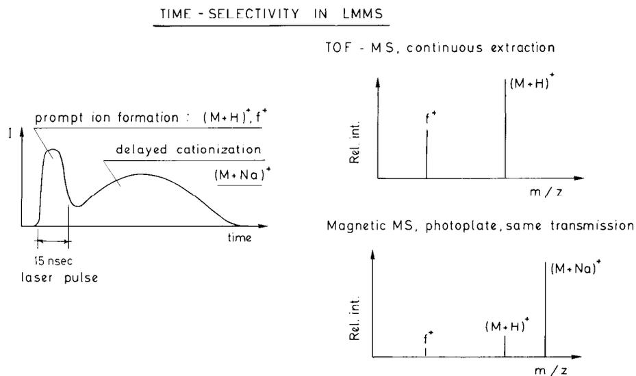
**Fig. 2.** Time selectivity of LMMS instrumentation compared with that of a magnetic instrument with photoplate detection for delayed ion formation
