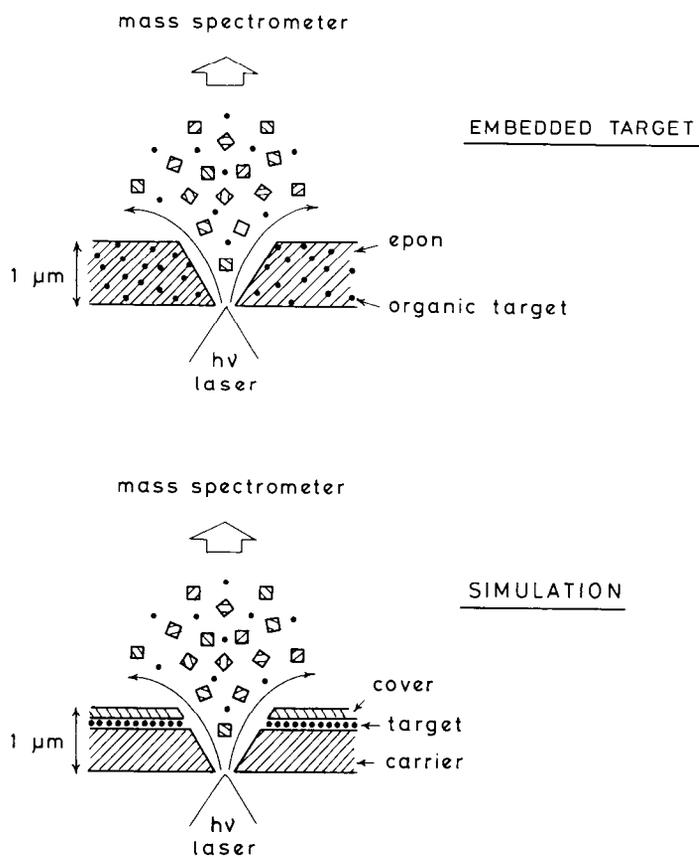
**Fig. 7.** Model sample simulation for the analysis of embedded targets by LMMS, and definition of carrier and barrier layers
